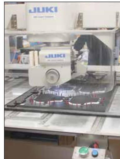
This CNC sewing machine is used to stitch the seats made at Mustang Motorcycle Products in Palmer.
